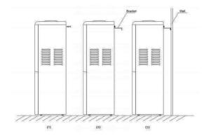
the screw already, fix the bracket tightening this removed screw on the right location (Picture 2).
