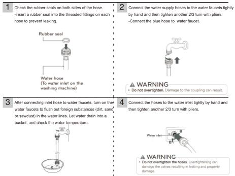
Check for leaks by turning on the faucets. If water leaks, check steps 1 to 4 again.
