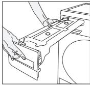
Drain the water in the tank.
