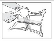
Clean the entire inner surface of the loading door and loading door gasket with a soft damp cloth.
