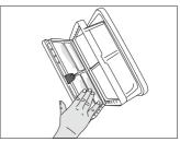
Wash the filter drawer sponge by hand to remove the fiber and lint on the surface. After washing the sponge, squeeze it by hand and remove the excess water. Well-dry the sponge before storing it.
