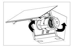
Place the lug slots of your new carbon filters into the lugs on the motor holder and turn them clockwise to snap them into place.
