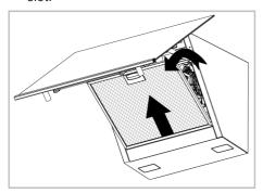
Reinstall the aluminium filter in its slot after flushing by following the above steps in reverse.
