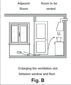
3. Intensive and prolonged use of the appliance may necessitate supplemental ventilation, e.g. opening a window or increasing the power of the air intake system (if present)
