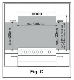
Should be cooktop be installed directly under a cupboard, later should be at least 720 mm (millimeters) from the top, as shown in Fig. C. The dimensions of the cutout for the appliance must be those indicated in the figure D. Clamps are provided to fasten the cooktop to counters measuring from 20 to 60 mm in thickness. To fasten the cooktop securely, it is recommended that all the clamps be used.
