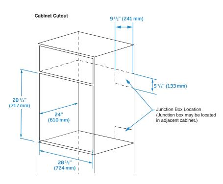
If installing in lower cabinet, leave 4" (102 mm) minimum clearance below.
