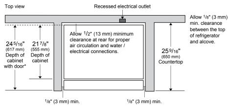
\*Dimension may vary based on panel thickness and door handle design (panel ready model only)
