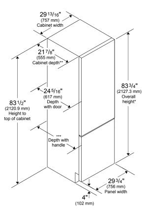
\*Add 1" (25.4 mm) with front leveling feet fully extended \*\*Add 1 3/4" (44.4 mm) for spacers on back
