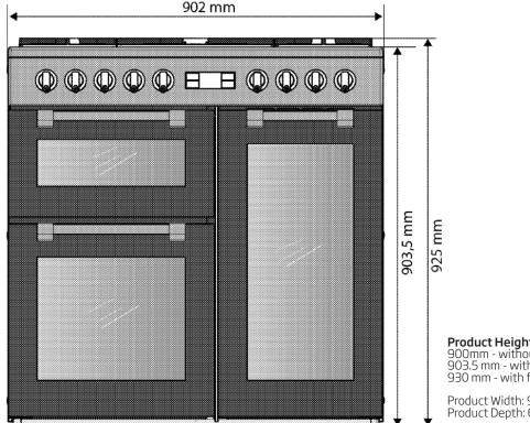
**Product Height** 900mm - without feet 903.5 mm - with feet fully tightened 930 mm - with feet fully open
