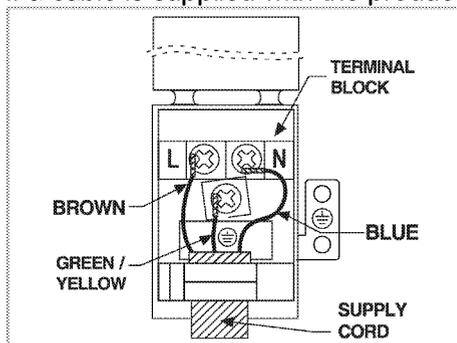
2. For single-phase connection, connect as identified below:
