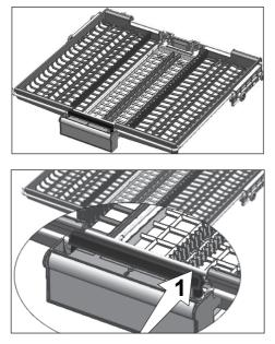
In models with partial movement feature, pushing the bar (1) on the handle enables the central tray of the basket to get to the lower position and the system gets unlocked. Thus right and left side trays can be used as moving parts.
