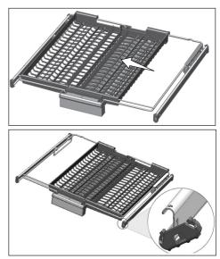
When the central tray is in the lower position, you can load long/high items such as coffee cups, ladles, etc. on the tray. When the side trays lean on two side walls, the handle can be pulled to allow the central tray to rise and the system to be locked.
